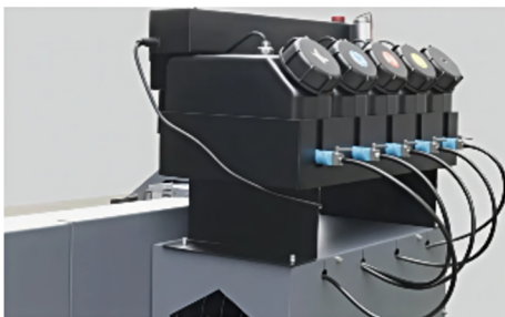
Ink shortage alarm + white ink stirrer Intelligent ink supply system to ensure the smoothness of printing
