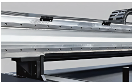
Imported guide rail THK silent guide, more smooth, higher printing accuracy
